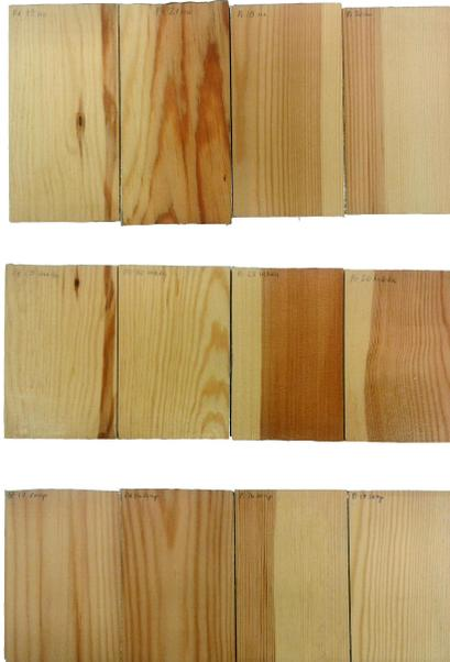
**Figure 1** Tangential (left) and radial surfaces with untreated (top), varnished (middle) and soap treated (bottom) pine boards were exposed to cycling humidity conditions. Five sides of the boards were sealed with aluminum tape. Species from left: ash, birch, black alder, elm, maple and oak.
