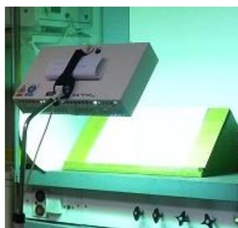
**Fig. 4** UV+IR quartz lamp
