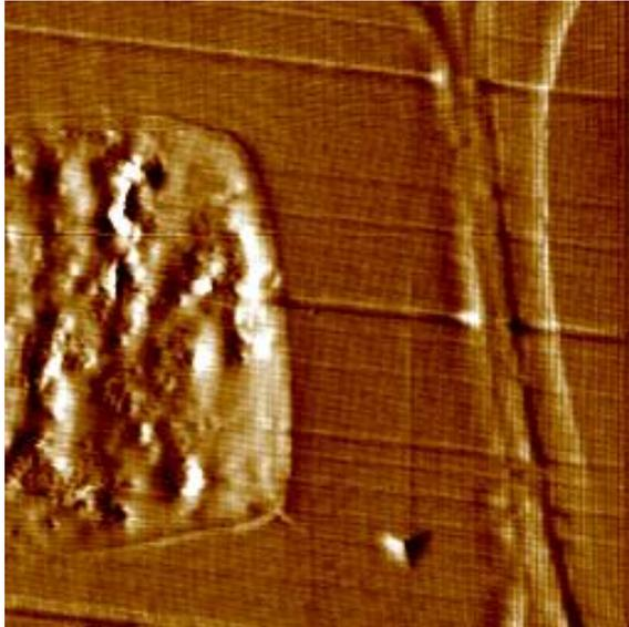
**Figure 2-3: Example of an indent for cell wall characterization.**
