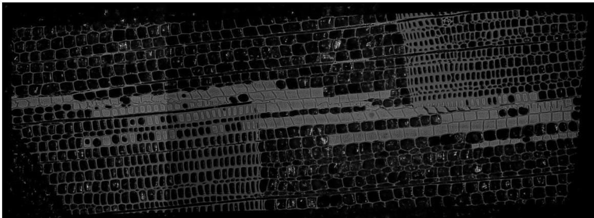
**Figure 2-2: Microscopic mapping of the bondline, magnification 100x.**
