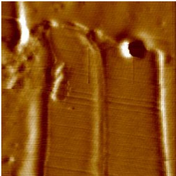
**Figure 2-5: Location of nanoindents for quantification of adhesion of S2 and adhesive.**
