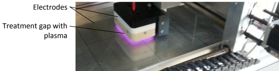
**Figure 2-1: Equipment for plasma treatment.**
