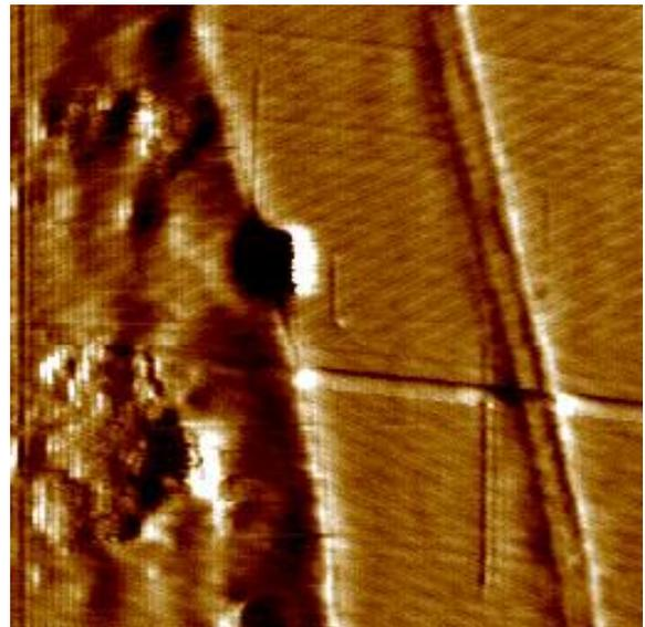
**Figure 2-6: Location of nanoindents for quantification of adhesion S3 and adhesive.**
