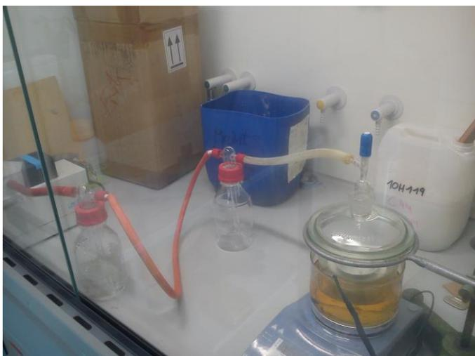
**Figure 2. Gas state esterification setup**
