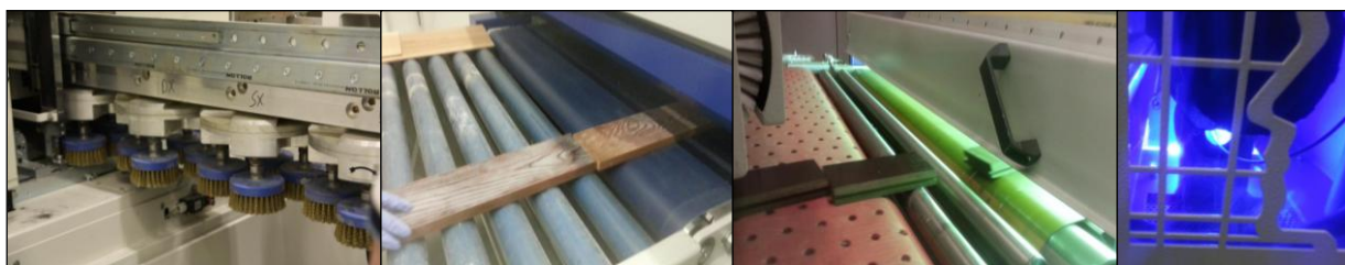
Figure 1. Stages in industrial coating process. From left to right sanding, applying, curing and Mercury lamps
