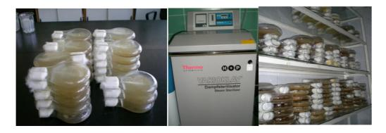
Additionally, a mixture of microfungi species were tested, in order to determine the impact of the treatments on surface durability of the specimens. The spore suspension for the microfungi species was the following: *Aspergillus niger* (An), *Trichoderma viride* (TV), *Penicillium funiculosum* (Pf).
