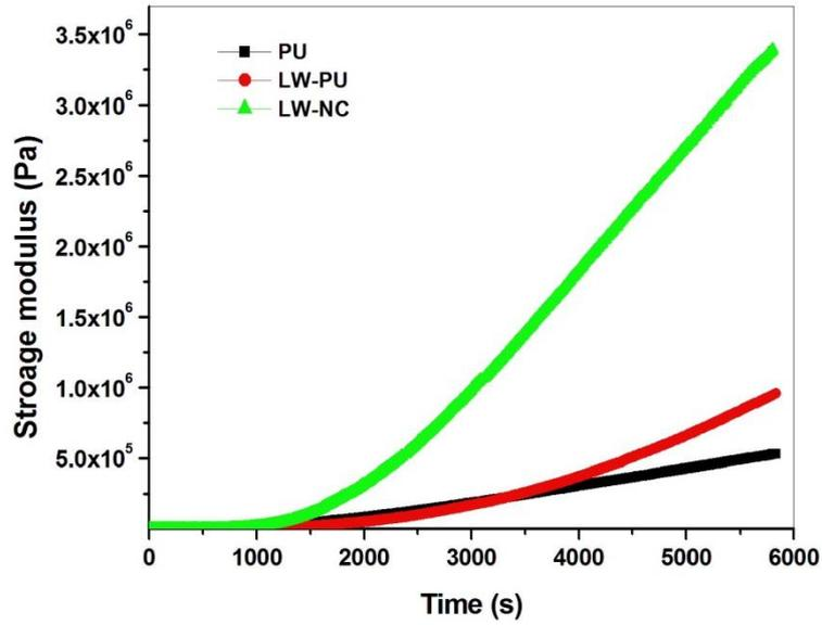
**Figure 3:** Storage modulus of all three types of polyurethane samples at 80 °C for 90 minutes of curing.
