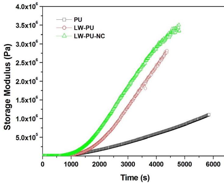
**Figure 6:** Storage modulus of all three types of polyurethane samples at 100 °C for 90 minutes of curing.
