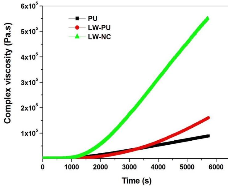
**Figure 5:** Complex viscosity of all three types of polyurethane samples at 80 °C for 90 minutes of curing.
