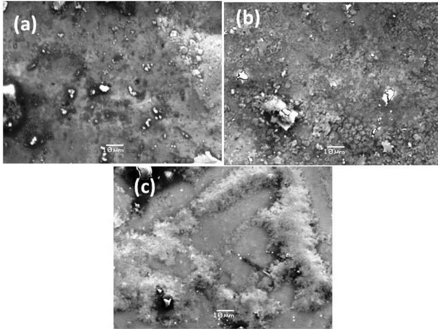
**Figure 2:** Nanosilica deposited on LW coated wood samples with three different concentrations of nanosilica in the solvent.
