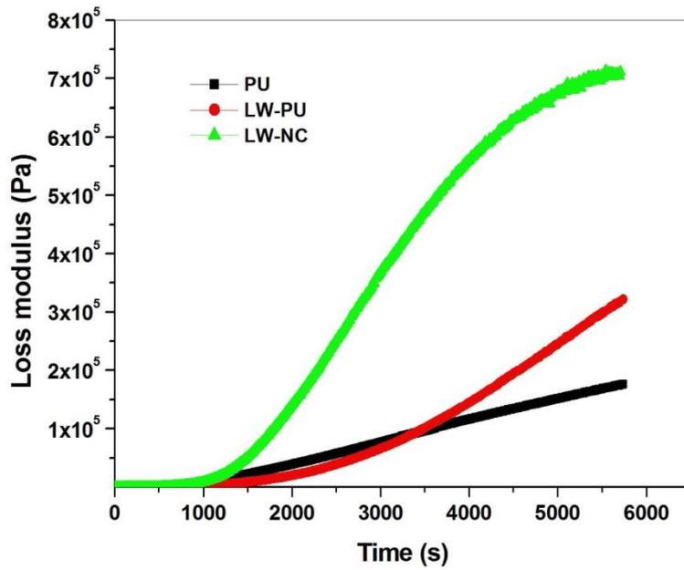
**Figure 4:** Loss modulus of all three types of polyurethane samples at 80 °C for 90 minutes of curing.
