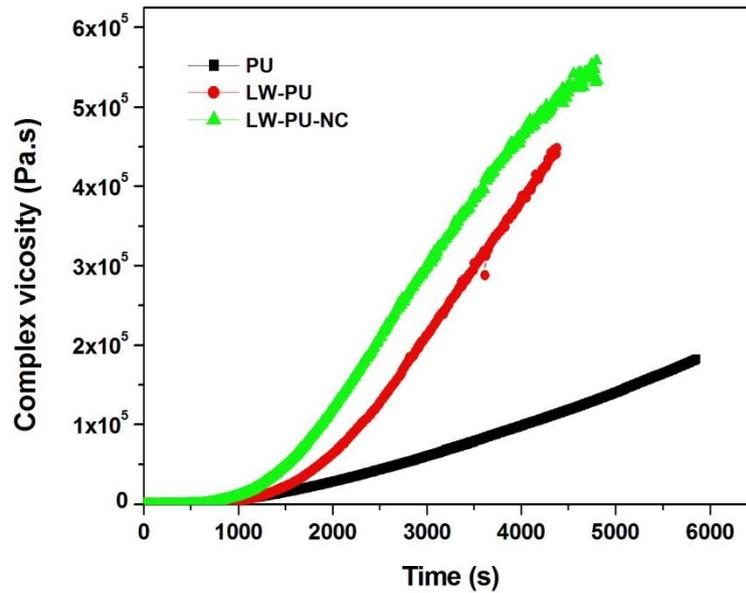
**Figure 3:** Complex viscosity of all three types of polyurethane samples at 100 °C for 90 minutes of curing.
