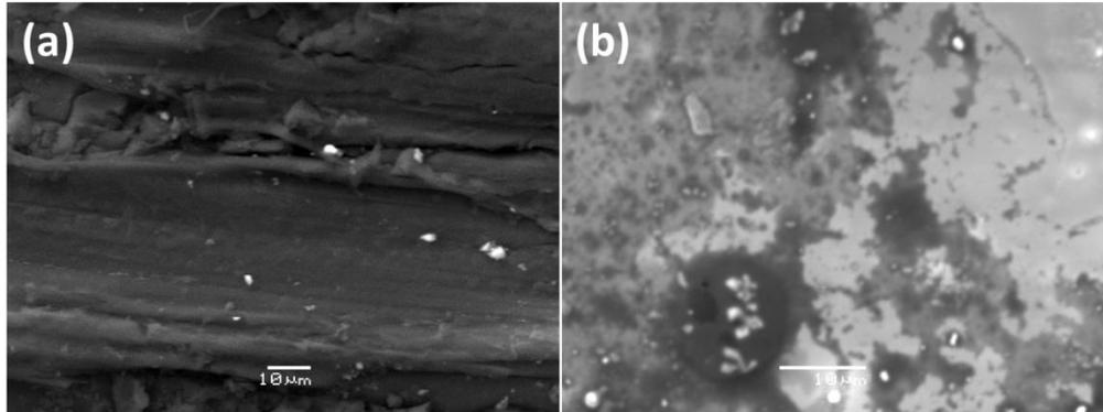
**Figure 1:** SEM images of (a) spruce wood and (b) LW coated spruce wood.
