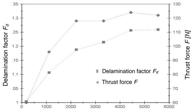
Figure 2. Dependency of delamination factor  $F_d$  and maximum thrust force  $F$  of drilling from the number of drilled holes
