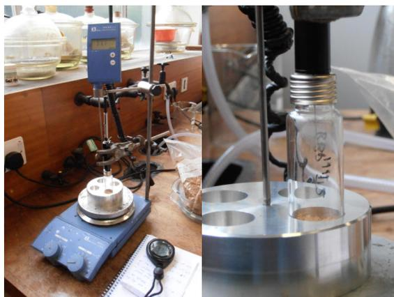
Figure 2: Sampling apparatus (left). Detail of the vial in the temperature controlled platform with DVB/CAR/PDMS fibre during sampling (right).
