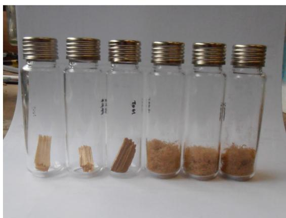
Figure 1: Wood and fibre samples in headspace vials.
