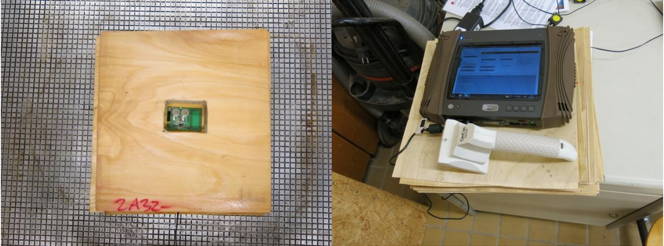
Figure 2. On the left an Easylog chip placed into a hole cut to a lay-up. Before putting the lay-up into the press several surface veneers were placed above the lay-up shown. On the right the reader and a tablet for controlling the measurement and collecting the data after reading it from the chip.
