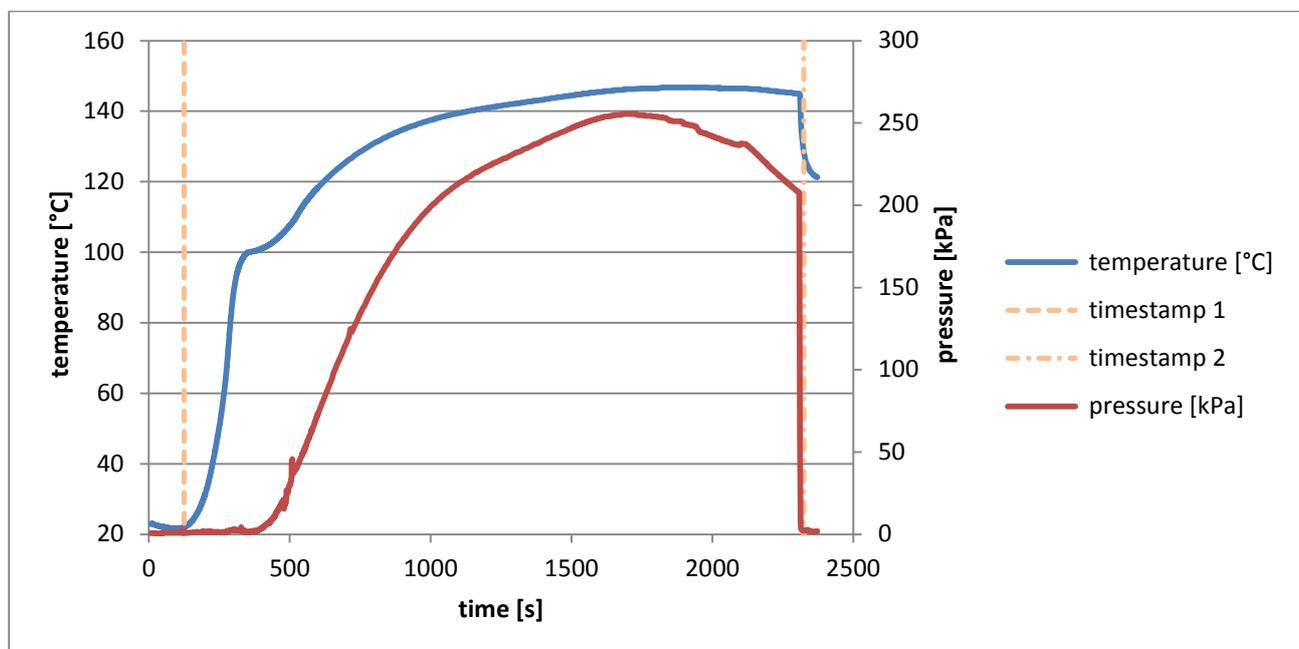
Figure 3. Red line shows the internal gas pressure and the blue line the temperature, both in the core part of the lay-up.
