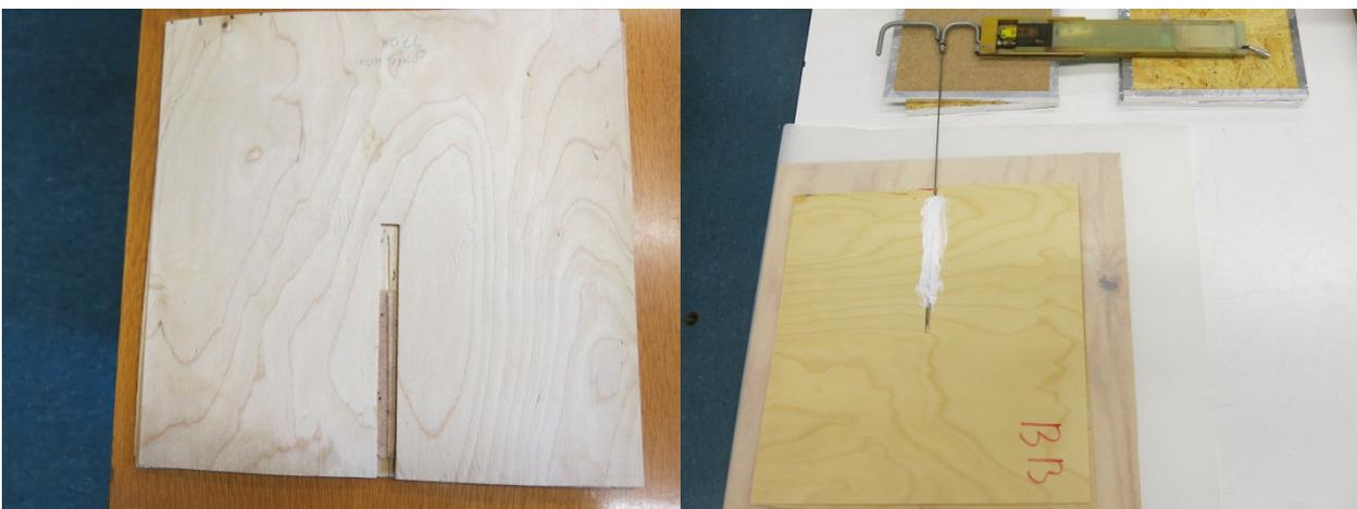
Figure 1. Pressman with a 300 mm steel tube and sealing with both MDF fibres (left) and silicone (right).
