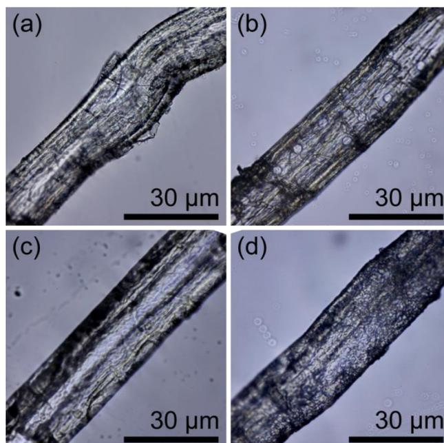
Figure 9: Light micrographs of (a)  $Ref_w$ , (b)  $^PRef_w$ , (c)  $^LPTMOS_w$ , (d)  $^{PL}PTMOS_{KPF}$  Kraft-pulp fibres.
