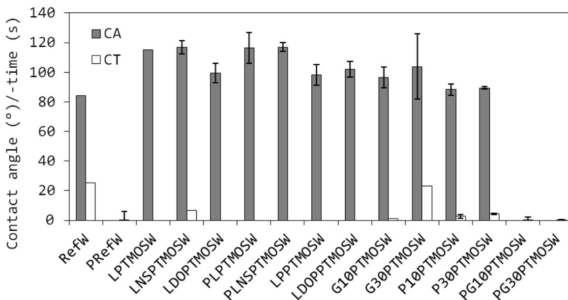
Figure 3: Contact angles and -times of the treated wood pieces named in Table 1, showing that high contact angles were obtained by plasma activation and solventless impregnations.
