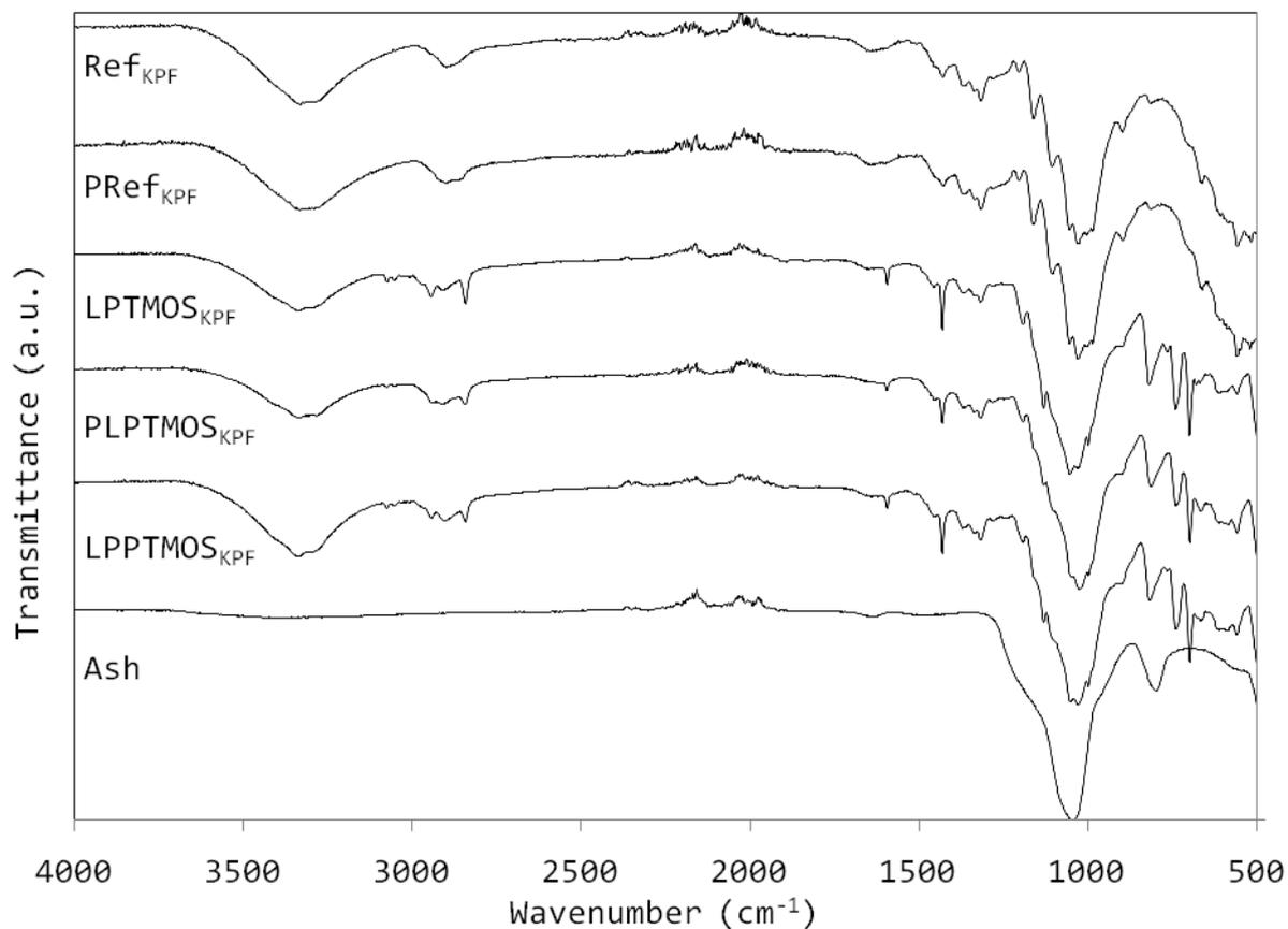
*Figure 8: Infrared absorption spectra from Kraft-pulped pine wood fibres showing the inclusion of phenyl groups, silicon oxide compounds and the effect of plasma activation and curing by the removal of absorption bands assigned to methyl groups compared to  $^{\text{L}}\text{PTMOS}_{\text{w}}$ .*
