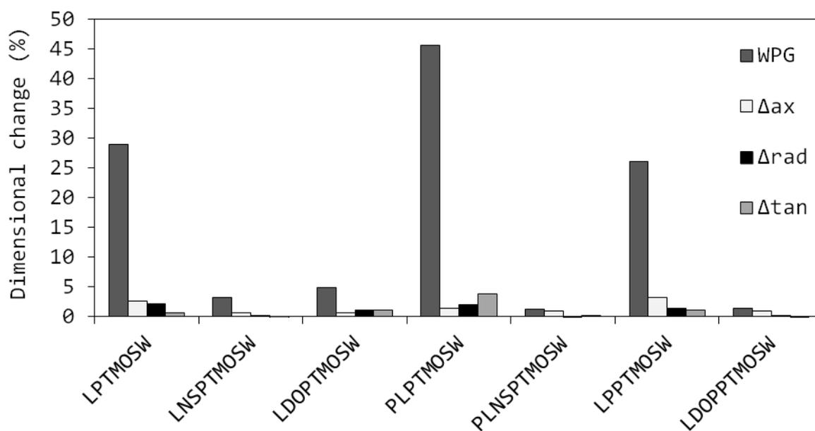
Figure 4: Dimensional changes of treated wood pieces showing that drying in the precursor solution results in the largest mass and volume increases during treatment.
