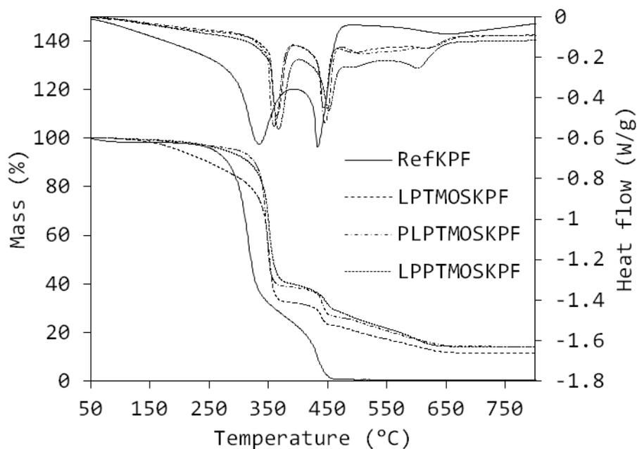
Figure 7: Thermal analysis curves of native and treated pine wood fibres showing the increased temperature resistance of all treated samples and the increased degree of precursor condensation imparted by both plasma activation and curing. Negative heat flow values indicate an exothermic process.
