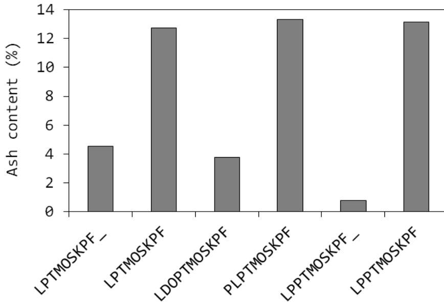
Figure 6: Ash contents of treated Kraft-pulped wood fibres showing that the total amount of deposited precursor is similar for all liquid impregnations dried in the precursor solution. Experiments followed by an underline were conducted on pulp aggregates.
