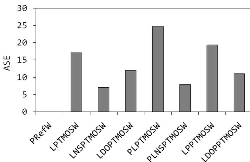
Figure 2: ASE of the treated wood pieces, illustrating the increased effectiveness of plasma pretreatment. Samples that were cracked from drying stresses are named, but results omitted.
