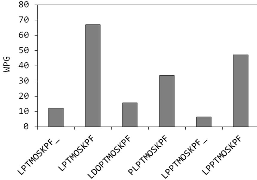
Figure 5: WPG of treated Kraft-pulped wood fibres, showing varying mass increases during treatments. Experiments followed by an underline were conducted on pulp aggregates and illustrate the need for well-dispersed fibres to achieve high deposition rates.
