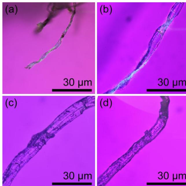
Figure 10: Polarised light micrographs with a 535 nm compensator of (a) Ref<sub>W</sub>, (b) <sup>P</sup>Ref<sub>W</sub>, (c) <sup>L</sup>PTMOS<sub>W</sub>, (d) <sup>PL</sup>PTMOS<sub>KPF</sub> Kraft-pulp fibre ashes.
