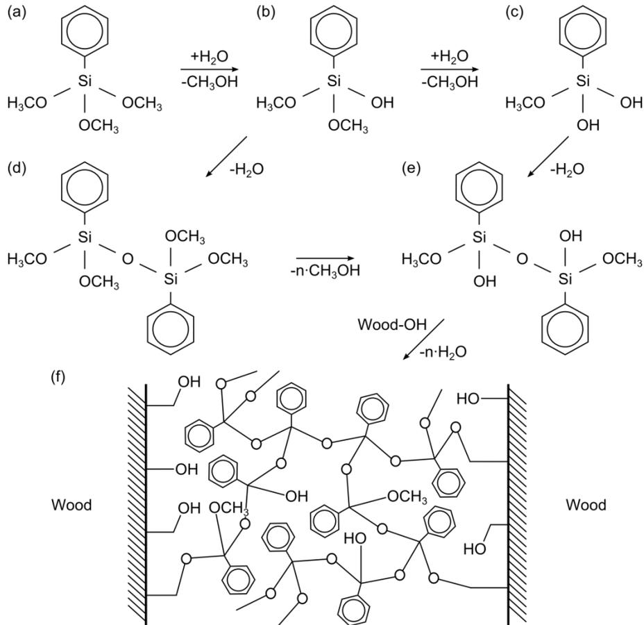
Figure 1: (a) Phenyltrimethoxysilane and its (b) single or (c) multiple hydrolysed forms condense under loss of water either (d) immediately or (e) after further hydrolysis. Condensation with wood hydroxyl groups, forming (f) a network under loss of water, has been shown to occur. This network is formed between the cellulose fibrils in the cell walls, preventing water uptake [2].
