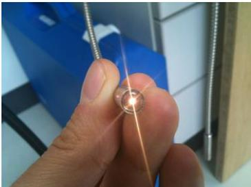
**Figure 4.** GetSpec in-line colorimeter sensor
