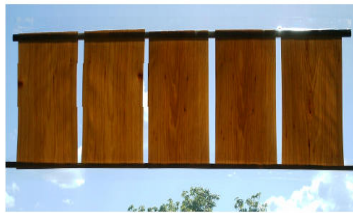
Trial stand for indoor sunlight exposure
