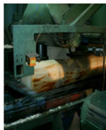
Figure 2. Freshly cut alder veneers: debarking of alder log (a), prism cutting (b), vertical slicing machine (c).
