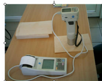
Figure 4. Veneer sheet (a), CIE Lab Colour space (b) and Chroma Meter Konica Minolta CR 410 device (c).
