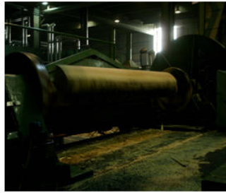
Figure 3. Half-round slicing for alder veneers (a) and flat slicing for cherry veneers (b) when using thermally treated logs (60-70°C for 10-12 hours).
